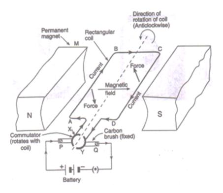
Initially, the coil ABCD is in the horizontal position. On pressing the switch, current enters the coil through carbon brush P and commutator half ring X. The current flows in the direction ABCD and leaves via ring Y and brush Q. The direction of magnetic field is from N pole to S pole of the magnet. According to Fleming's left-hand rule, the force on sides AB and CD is in the downward and upward directions respectively. This makes the coil ABCD move in the anticlockwise direction.
