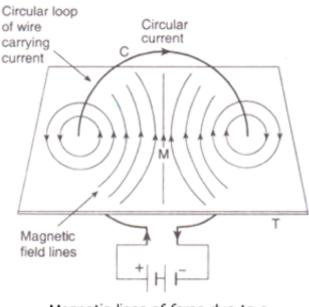
Magnetic lines of force due to a circular wire carrying current
