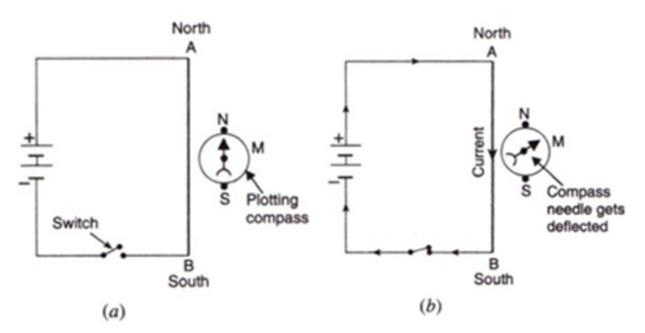
let us take a copper wire AB on a plane such that it faces North-South. Now place a plotting compass under it. connect both end to a battery with a switch to put it on and off.
