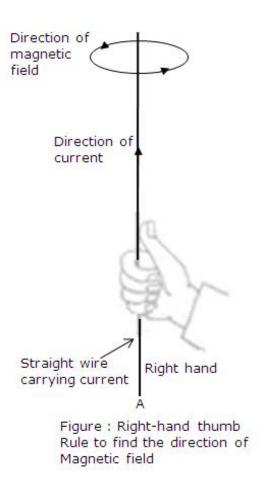
Let AB be a straight wire. Placed vertically A to B. To find the direction of magnetic field we assume that we are holding the current carrying wire in such a way that our thumb of right hand shows the direction of flow of current. Then the finger enclosing the wire. The direction in which our finger is enclosed shows the direction of magnetic field which is anticlockwise.
